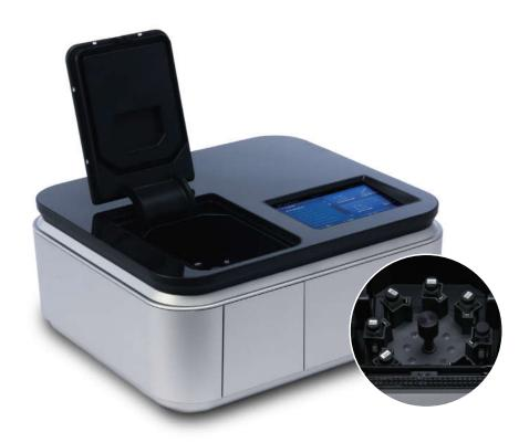
OPTIZEN POP offers four measurement modes (Photometric Mode, Quantitative Mode, Spectrum Mode, Kinetics Mode). The user can choose a suitable mode depending on the purpose to measure. The embedded S/W, touch screen interface and application facilitate the use of the device.
