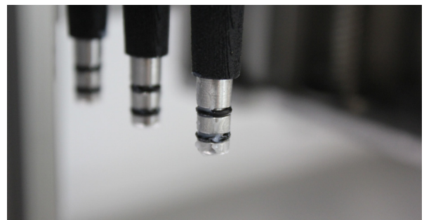
Too much grease
