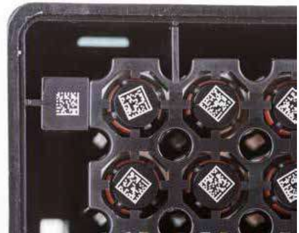
2D coded rack base allows automatic detection of orientation by instrumentation
