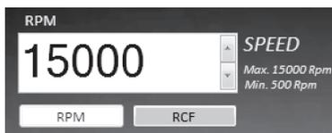
Click on **RPM** or **RCF** button to read speed value in RPM or RCF mode for active line.
