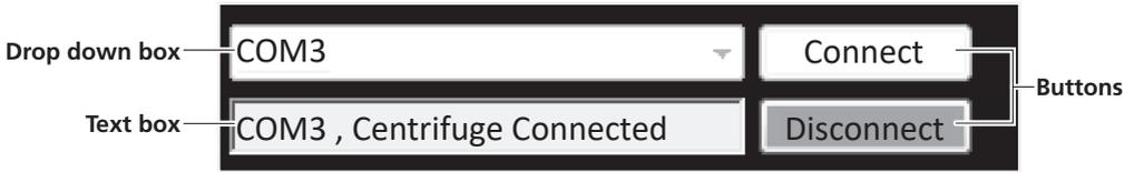
Once you connect the USB cable, the Com port for the centrifuge is detected automatically. Click on the **Connect** button to connect centrifuge and computer for remote operation. After connection, the **Text box** will show **COM3, Centrifuge Connected**.
