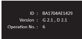
After the centrifuge has been connected, the centrifuge ID and version will display in the GUI screen. The operation number shows the number of operations performed using the software.
