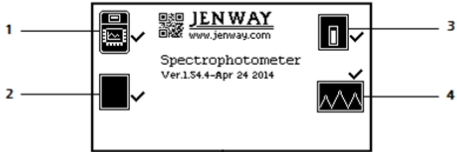
Fig 2.2.2 – All Power On Tests Complete
