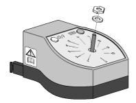
9.3.3. Turn the controller up-side down and remove the two fixing screws retaining the base.
