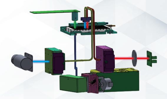
INNO-S<sup>™</sup> has three main detecting functions. Since INNO-S<sup>™</sup> is a monochromator-based microplate spectrophotometer for the absorbance measurements, it requires zero filters and allows you to measure from 200 to 999 nm freely at your choice of 1nm increment. Also Xenon lamps in absorbance will serve the instrument semi-permanent life time which brings the comfortable experiences to the users since the lamps do not need to be replaced such as halogen lamps.
