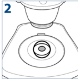
2 Put a specimen on the stage plate
