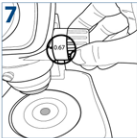
7 Turn the zoom adjustment knob to the lowest magnification
