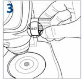
3 Turn the zoom adjustment knob to the lowest magnification
