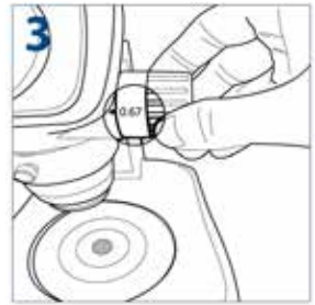
Turn the zoom adjustment knob to the lowest magnification
