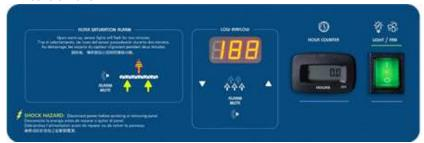
The controller displays the airflow and offers limited detection of low concentrations of hydrocarbon, some gases and organic acids. Audio and visual alarms alert users to filter saturation and if the airflow reaches preset thresholds. An Hour Counter with preset alarm intervals for pre-filter and main filter change out is also included.
