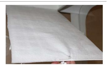
Open the sash and lift pre-filter tray into the inlet cutout. Rotate the wing nuts on each side to support the tray.
