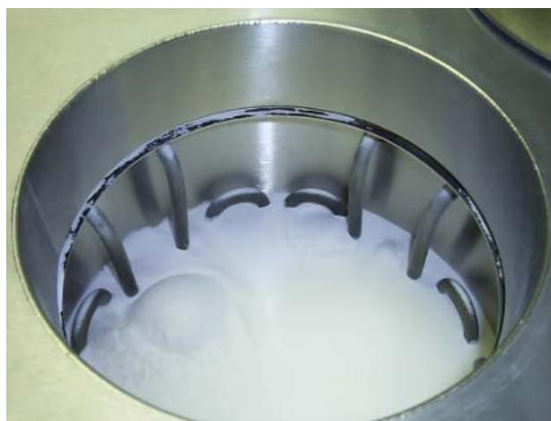
Figure 3: fluidized alumina at the correct operating level
