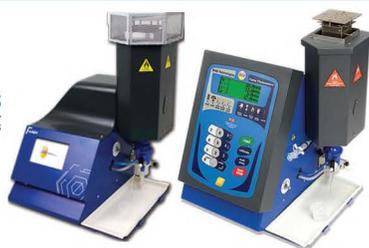
BWB Technologies (UK) have revolutionised what can be achieved using low temperature flame analysis. They are the first real alternative to AAS and ICP for measuring Lithium Li, Sodium Na, Potassium K, Calcium Ca & Barium Ba. BWB continues to develop and enhance flame photometer technology and accessories.
